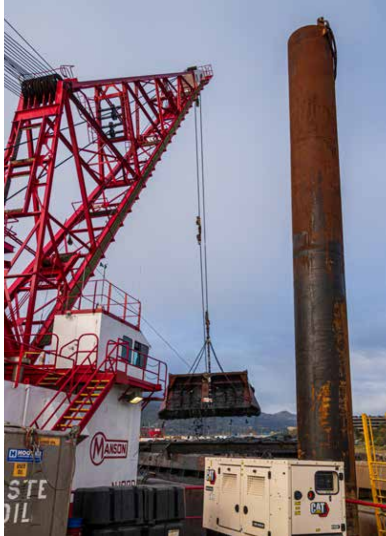
The bucket of the Njord holds up to 50 cubic yards, the equivalent of five dump trucks.
