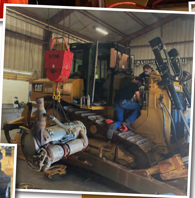
Students remove components off the D6T for injector repair.
