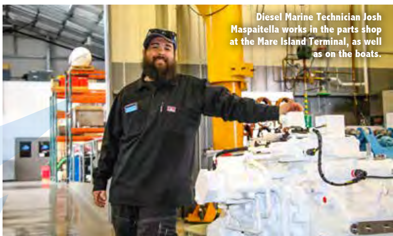
The new 16-cylinder Series 2,000 MTU engine is readied for placement on the Taurus.
