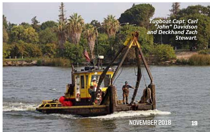
Dredge No. 8 uses a discharge pipe to collect unwanted material on the San Joaquin River bottom.
