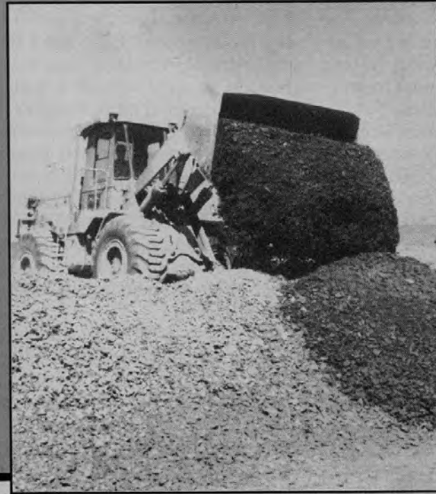
Left: Loader Operator Don James scoops the material and moves it to a storage area. This material later will be sold for use as road base.
