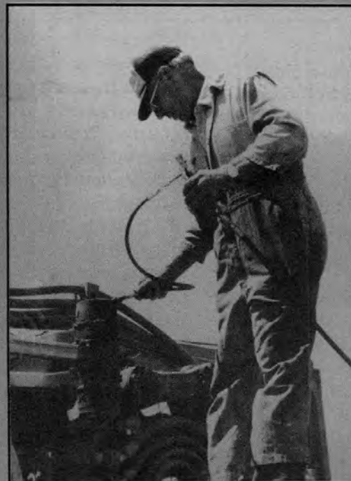
While the operators break for lunch, the lubemen move in to perform some preventative maintenance. Apprentice Lubeman Mike Gills (right) readies his lube gun, while Journeyman Lubeman Don Campbell (left) lubes a 631 scraper at the Shotgun Creek Project.
