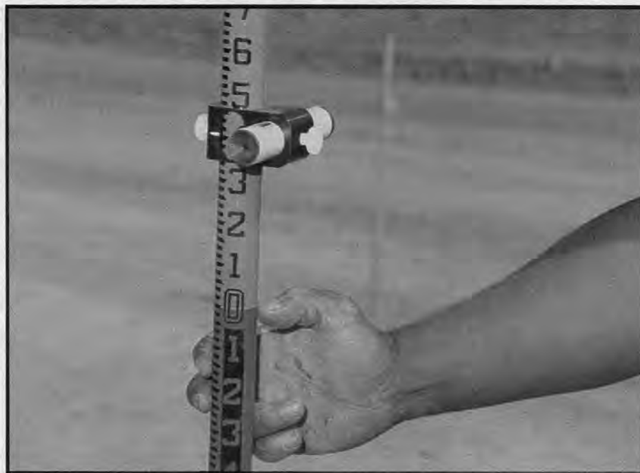
The Willie Rod has cut and fill graduations painted red and blue.
