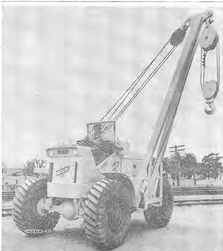
SIDE BOOM ATTACHMENT on a Michigan is shown here, designed and built for Buran Equipment Co. by Bro. Harry Livermore, Master Mechanic. Attachment has a capacity of 14 tons at 4 feet radius. Counterbalance is hydraulically controlled. Both boom hoist and load line can be powered up and down, or they can be lowered on the brake. Hoist system is made up of Carco standard logging winches. (Picture from Oakland office of Local 3).
