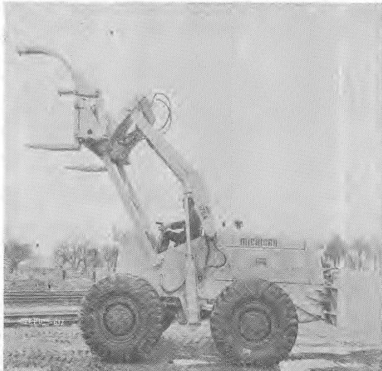
Powerful little log mover is this rig designed by Operating Engineer Harry Livermore of Oakland. It can pick up a nine-ton load and hold it in any position. (Picture, story from Oakland office.)
