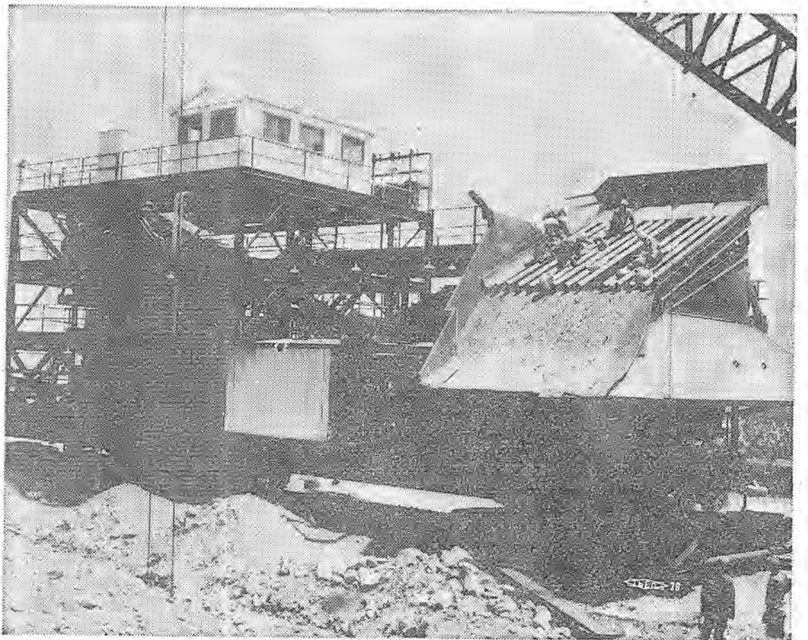
DRY LAND DREDGE . . . Here is a huge 380-ton machine put into operation by Utah Construction at Iron mine in Southern Utah. It is capable of 800 cubic yards per hour. Controls are in air conditioned cab on top. Machine has series of cobbles and magnetic head pulleys which separate ore from waste. It is fed by 8-yard Marion dragline.
