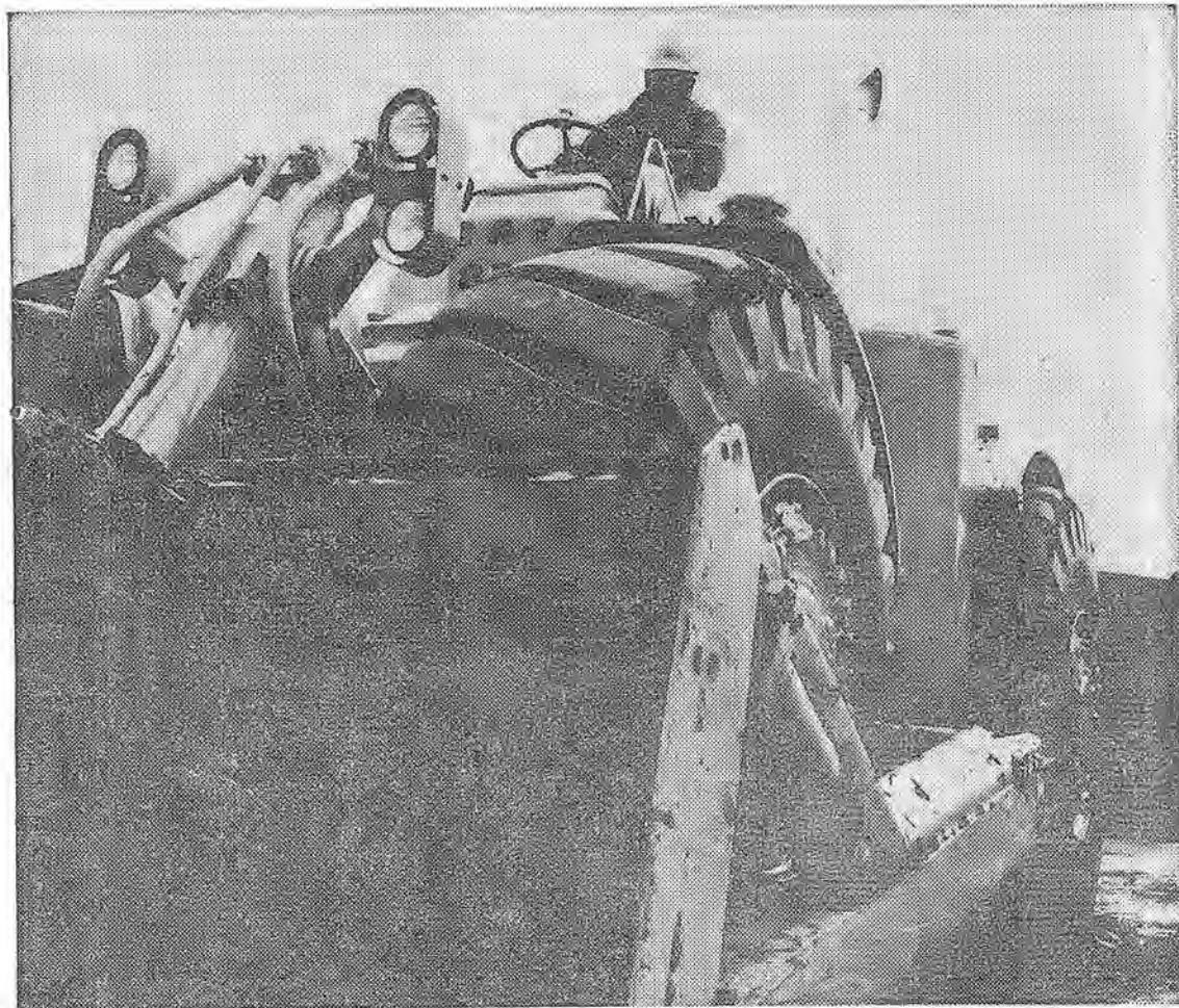
THE LATEST . . . Brother Pete Ramirez is proud of his 824 Cat pusher which has automatic drive, three speeds forward and back, power steering and hydra-lift. He's on the Green-Winston Dublin Freeway job in Alameda County.
