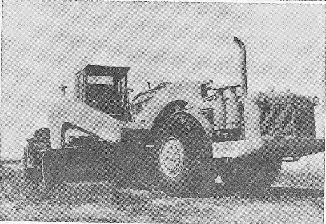
BIG EQUIPMENT . . . these two pictures show new equipment in use by Western Contracting Co. at its Del Puerto Canyon canal job in Modesto area, west of Patterson. Upper photo shows TTSS-40 Euclid twin scraper with three engines. Note size of equipment compared with car in foreground. Below is giant blade used on same project with enclosed cab.
