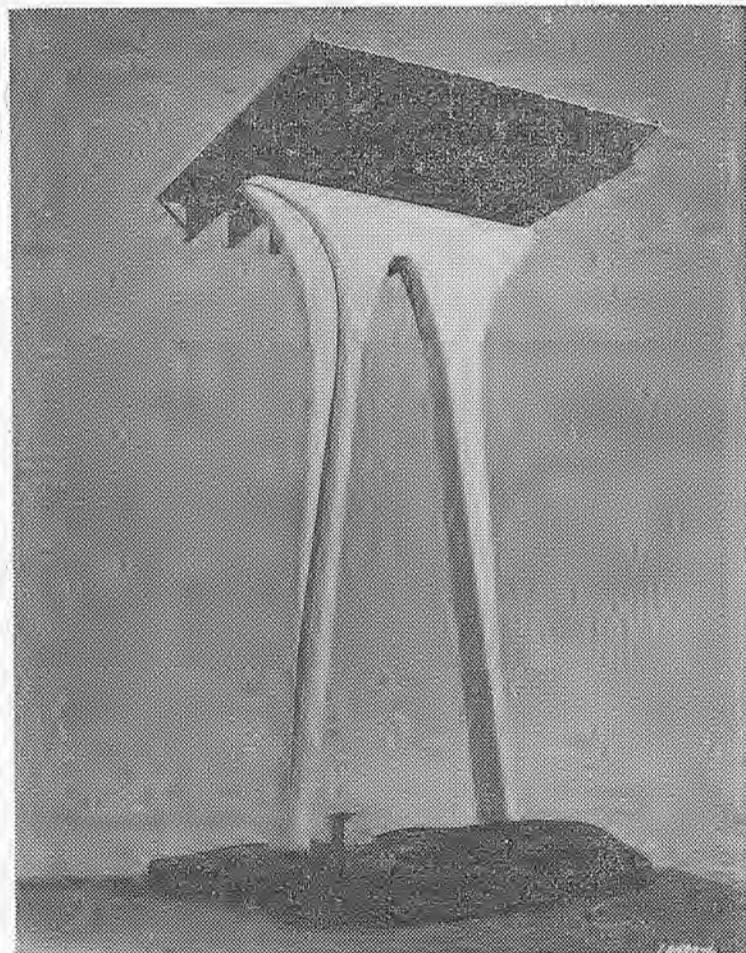
MODERN DESIGN . . . Supporting the five-span San Mateo Creek Bridge will be these specially-designed, tapered concrete columns, which rise as high as 250 feet above the canyon floor. Of modified Gothic arch design, the supporting columns will remain natural in color, with the steel superstructure to be painted green.
