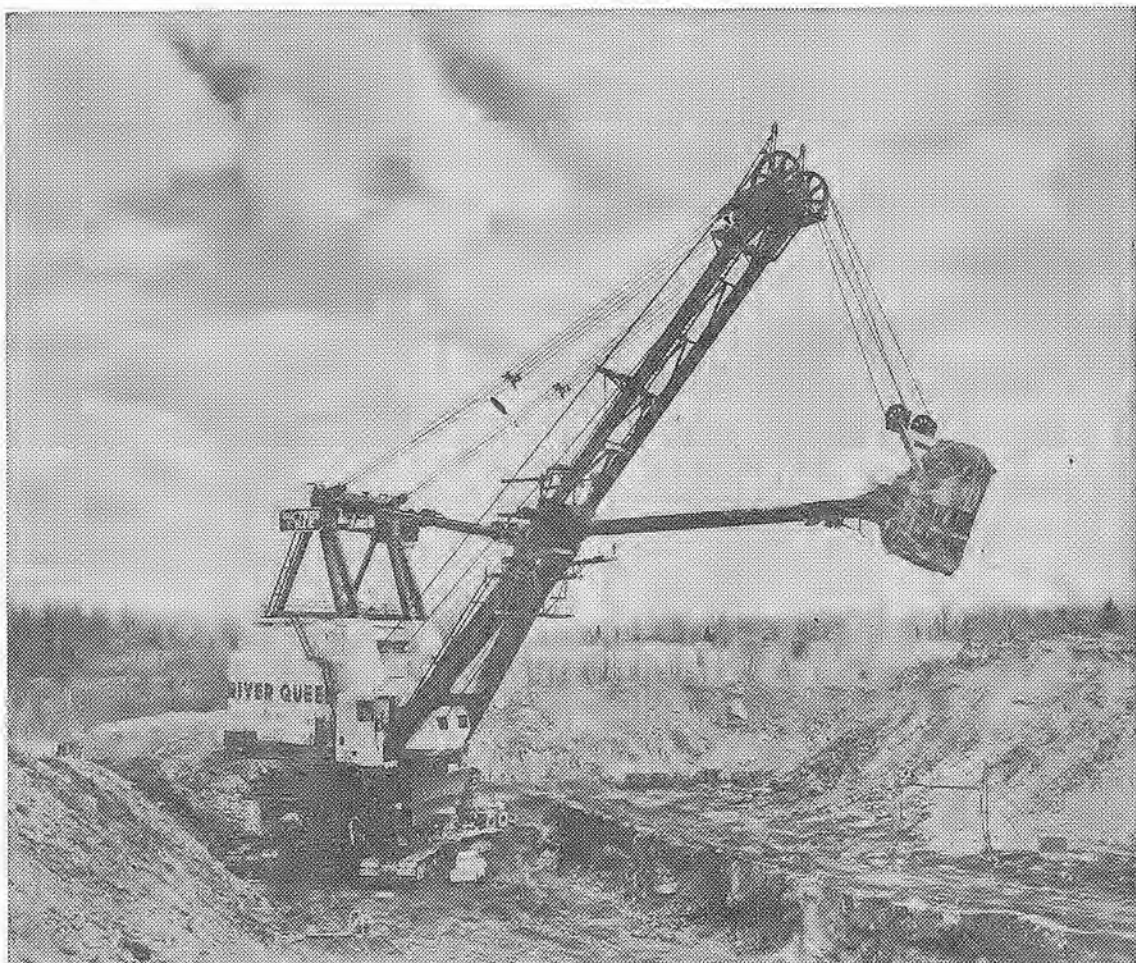
SWINGING SHOVEL . . . Standing on one seam of coal the "River Queen" clears overburden from an upper coal seam. Note how the pickup truck in the foreground and the bulldozer in the background are dwarfed by the machine. It has a 55 cubic yard bucket and its working weight is 4,850,000 pounds. It is the biggest coal-stripping shovel in the world and it is built by Bucyrus-Erie.
