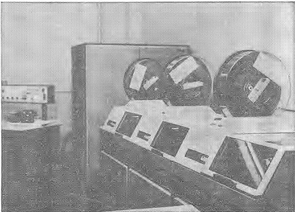
DISK DRIVES . . . this automatic data processing machine resembles a giant record player. On it is stored all membership records of Local 3. The central control is shown at the rear with the console at rear left.
