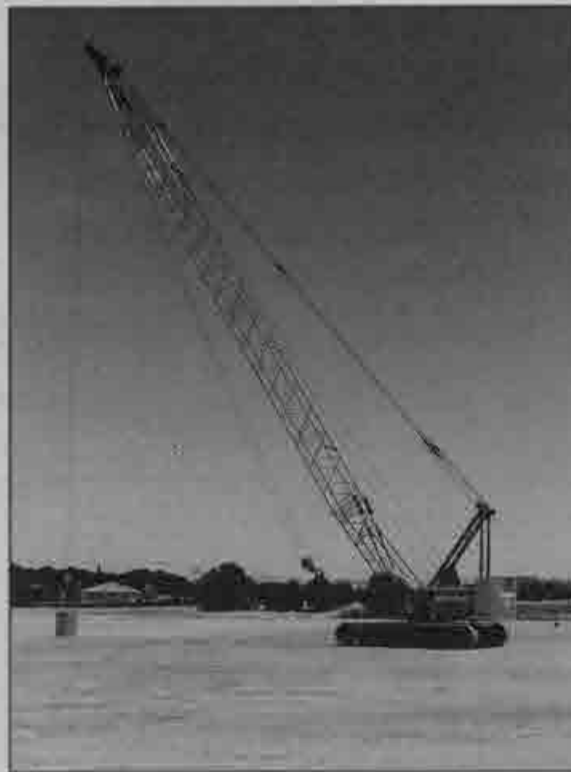
The training center's new Manitowoc 222 100-ton crawler crane.
