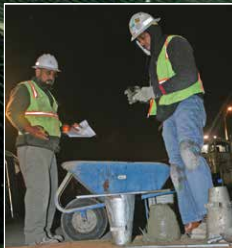
From left: Bedar Ahmed and Sherman Moore with Consolidated Engineering test the slump of the concrete.
