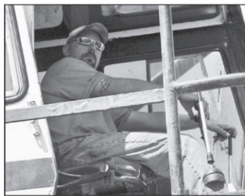
Dragline Operator John Stevens, an eight-year Local 3 member, uses precise timing to maneuver the dragline. With four hand levers and two foot pedals, operating the dragline can be a demanding job.
