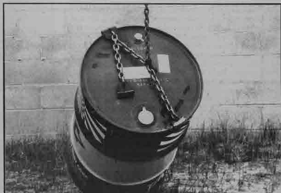
Right: The Riggitt also attaches to the top and bottom of the drum.
