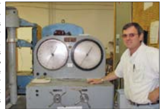
Local 3 Laboratory Technician Don Ensley uses this compression hydraulic machine, a Tinius Olsen model-L, to determine the compression strength of concrete. The machine can exert up to 300,000 pounds of compression force.
