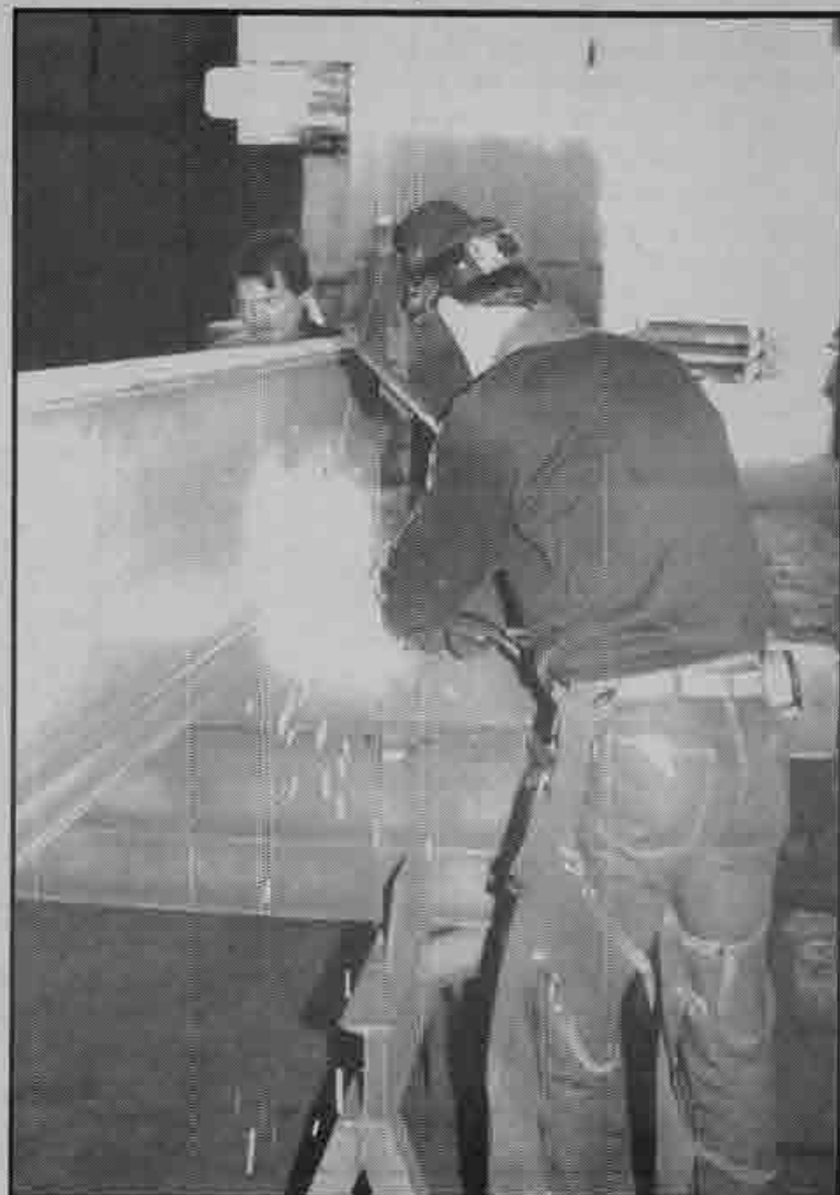
Below: Kent Schumacher applies a high-stress weld to the scale's main girders and cross members.
