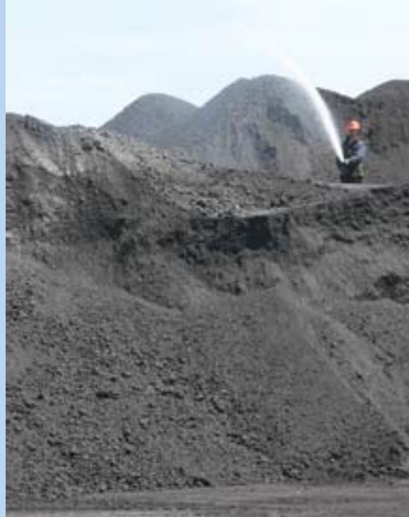
Arthur Warner hoses down the massive piles of petroleum coke at the Levin-Richmond Terminal to prevent it from blowing around the port.
