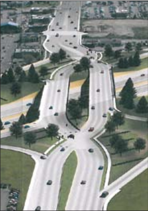
This is a conceptual drawing of the bridge and intersection being built at Main Street and I-15 on the Pioneer Crossing project.
