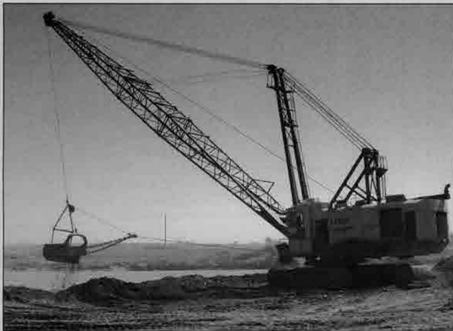
One-year Local 3 member Mike McAllister excavates material at the Marysville site with a Lima 2400B dragline.
