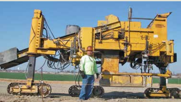
Member Hector Grimaldo uses the curb and gutter machine for Granite on the Mission Boulevard/Campus Parkway project off Hwy. 99.
