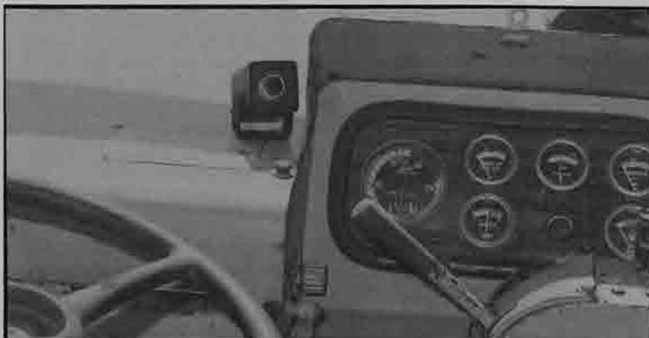
The warning light and buzzer installed near the main control panel alerts the operator that a stationary or moving object is behind the machine.
