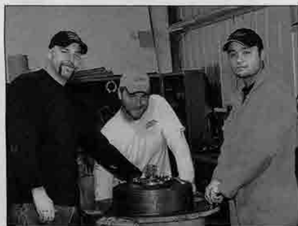
From left: Heavy-Duty Repairer (HDR) apprentices John Drouillard, Thomas Donoho and Endy Macheuca work on a 621 scraper transmission during a Power Train SRT class at Rancho Murieta.
