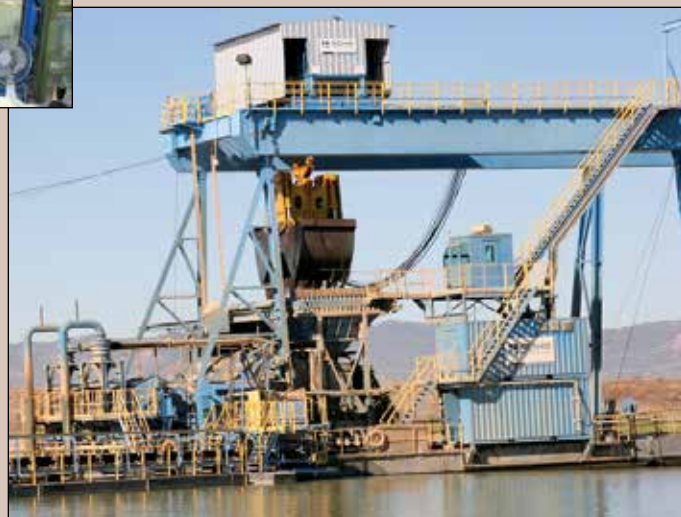
At the Rinker Materials Plant in Cache Creek, member Mike D'Aurizio operates the clam-shell dredge with a 20-yard bucket. He makes 320 loads a day or 7,000 to 8,000 tons of clay variable on a normal day.
