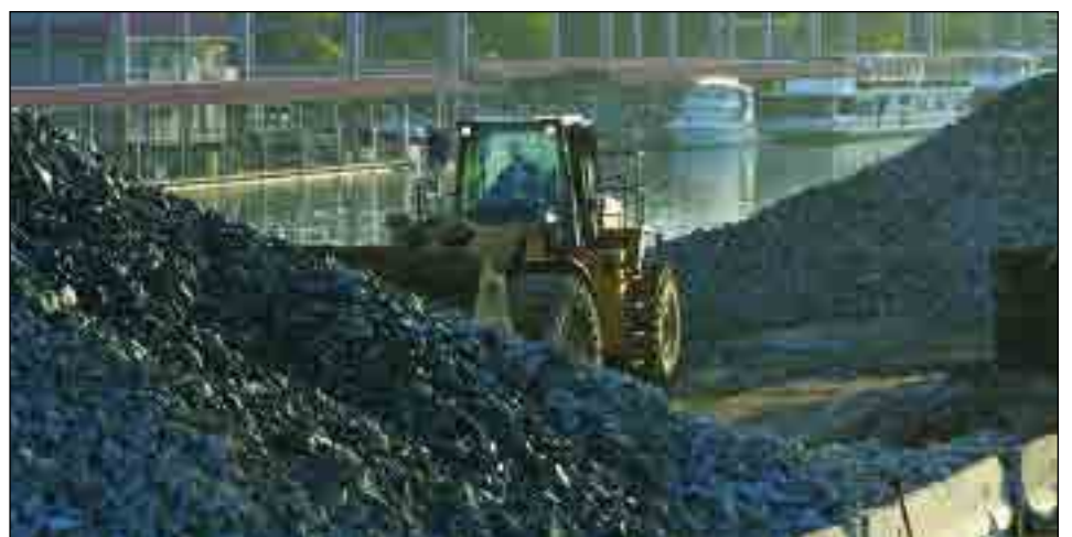
Rubber-tire Loader Mike Bledsoe loads an eight-yard bucket full of aggregate.
