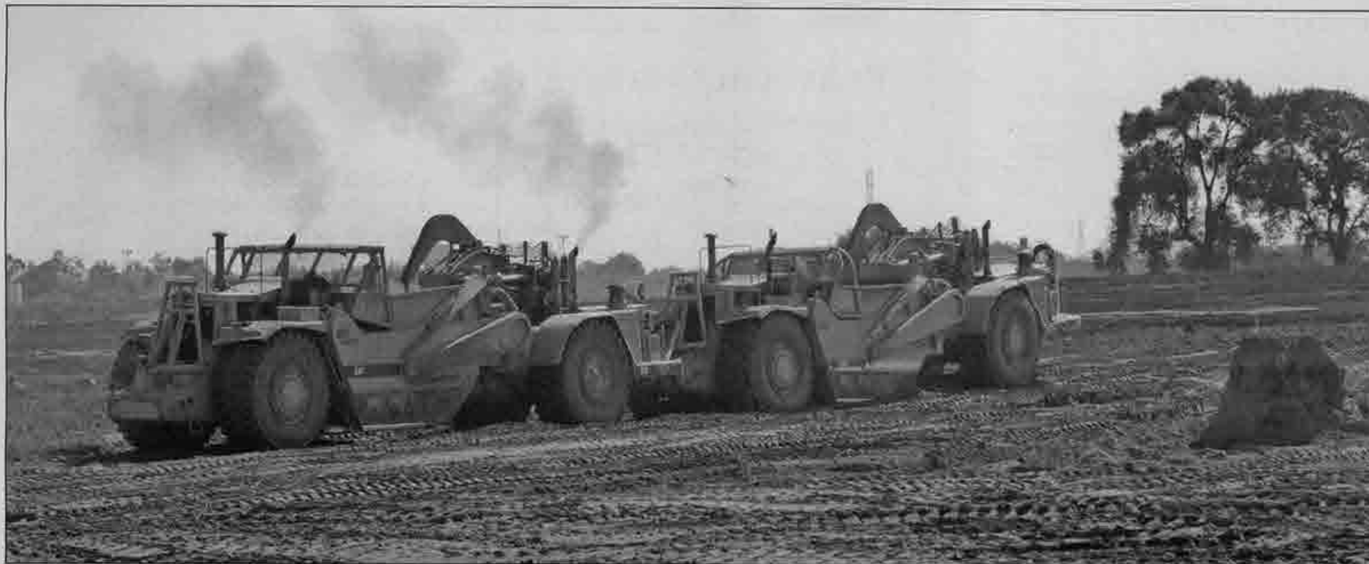
These scrapers operate in push pull to pick up large loads of dirt.
