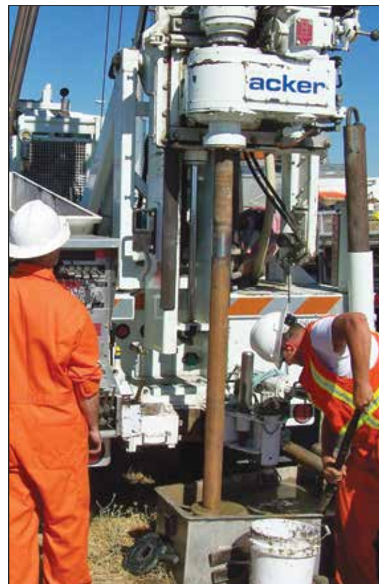
Caltrans members use an Acker MP8 drill rig to drill 125 feet while taking Standard Penetration Tests (STP) every five feet as part of the median bridge widening of the Winters Street Undercrossing in District 80.
