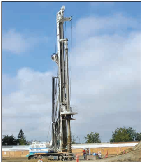
Pieces of equipment common to this Malcolm jobsite include a Bauer BG 18 drill, a Soilmec 725 drill, a concrete pumper and truck loader.
