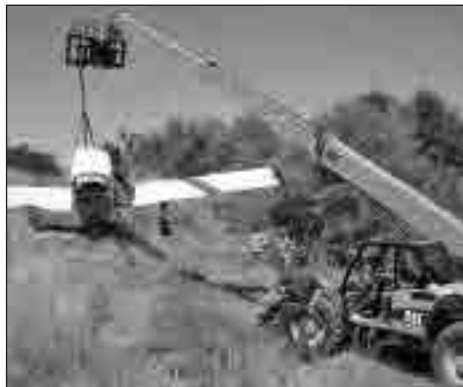
RMTC staff used this telescopic material handler to raise the airplane from the river bank and place it closer to the boom.
