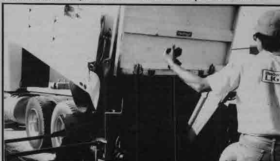
A conveyor belt moves the material out into the screed box, which can be adjusted for width and thickness.
