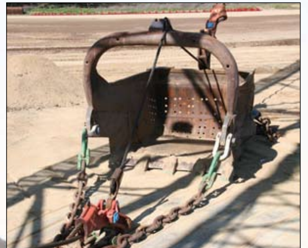
This 27-yard bucket is actually small compared to some of the dragline buckets on the market now. Even so, this bucket is responsible for the acquisition of all the rock, sand and gravel the Vulcan Materials plant needs.
