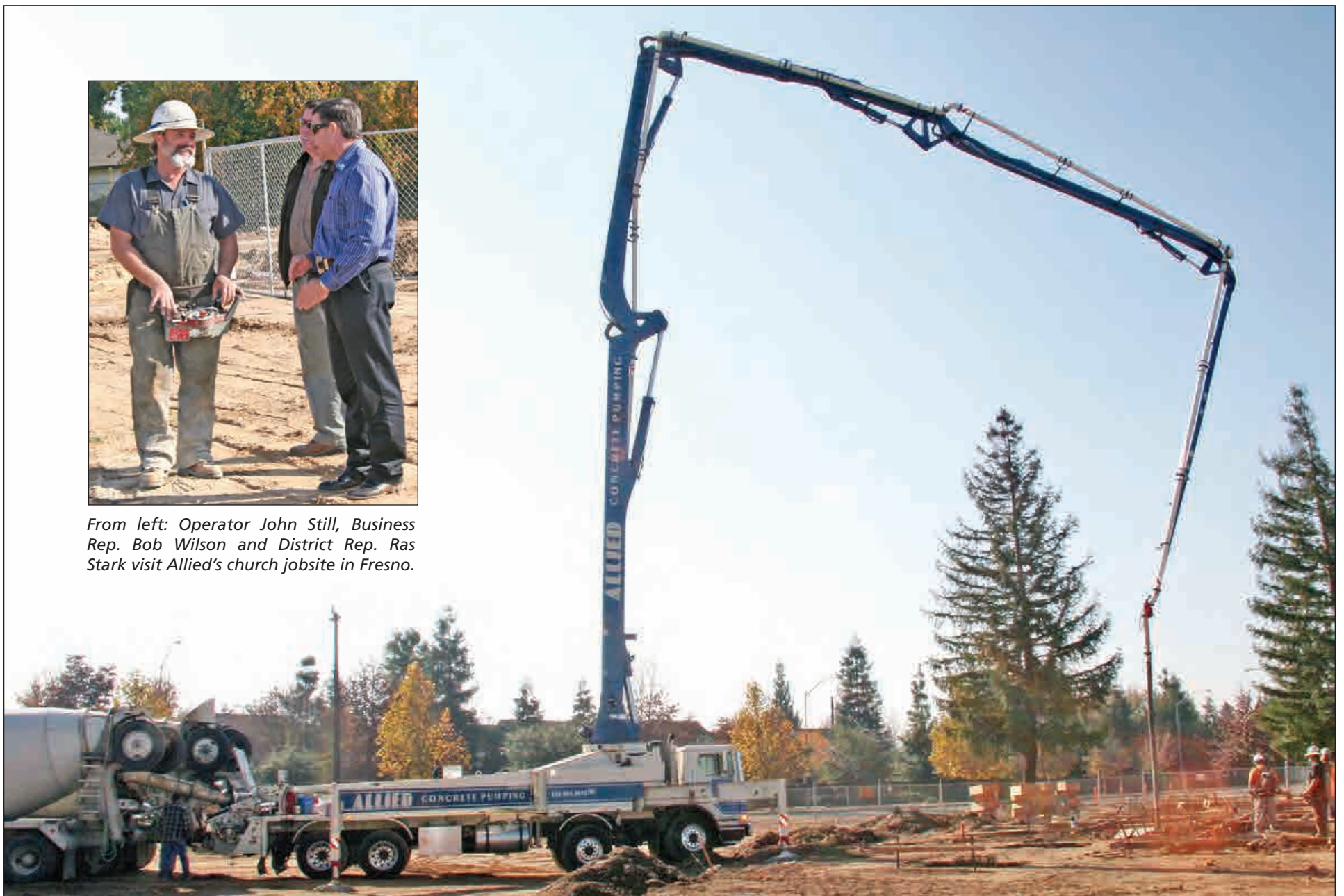
Local 3 member John Still operates this 47-meter truck-mounted concrete boom pump for Allied Concrete Pumping in Fresno.
