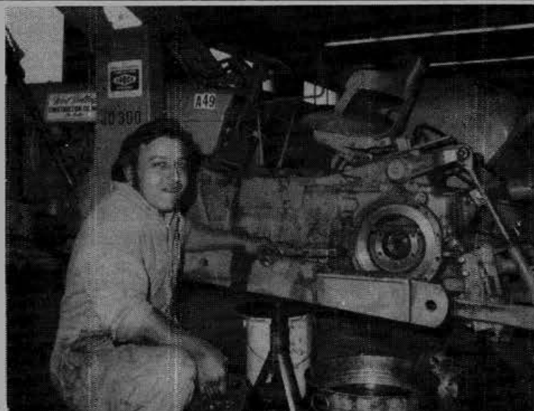
APPRENTICE ART FRECHOU repairs a broken axle on a wheel tractor. Frechou became a journeyman in March.
