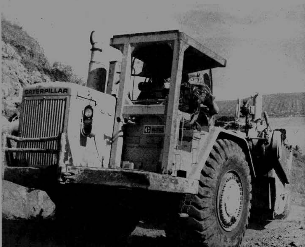
Member Herman Waa mans his CAT 631-C Scraper and works his way up the Hawaii Loa Ridge access road project. Other Local
