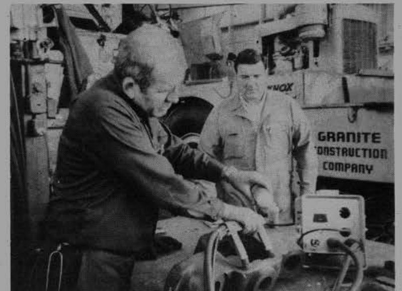
Granite Construction employee Dalton Fisher demonstrates the use of the new Magnaflux unit while Carl Serpa looks on.
