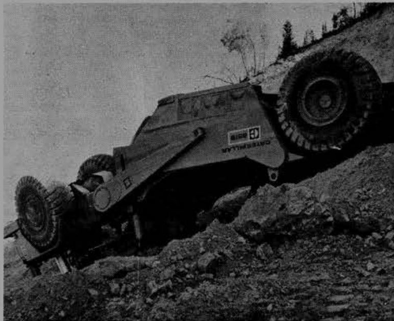
ROLLOVER PROTECTION prevented serious injury to the operator of this Cat 651-B scraper when it rolled over while working on the Currant Creek Dam project.
