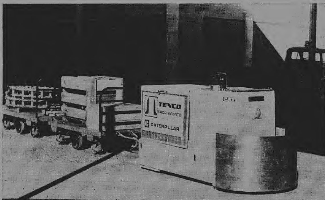
DRIVERLESS TRAIN is used by Tenco Tractor at its new facility to deliver a load of parts via outdoor covered concourse connecting six structures.
