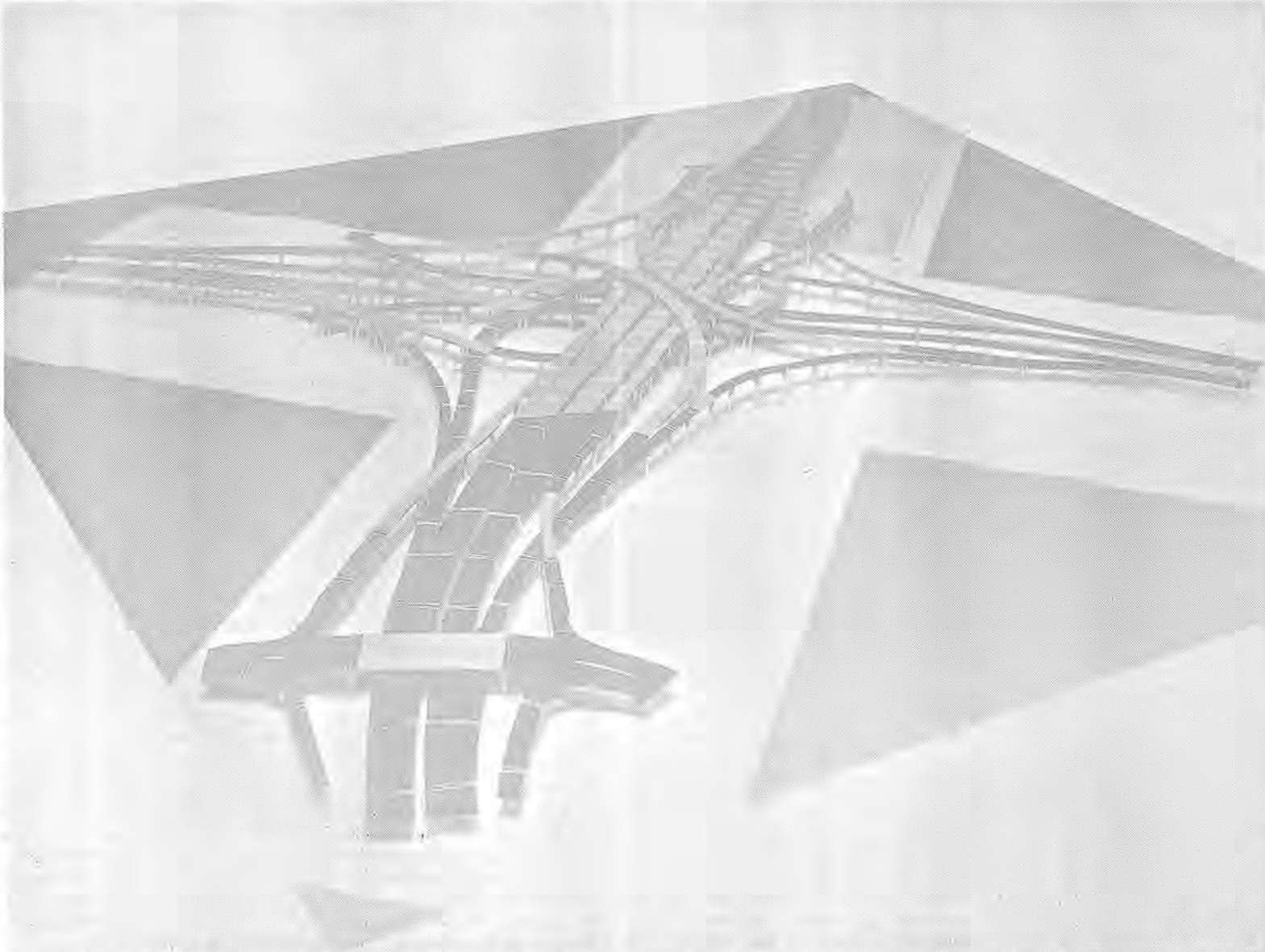
GUADALUPE FREEWAY complex in San Jose is shown in the model above. Granite Construction Co. was awarded the bid and work is expected to get underway late this month. The job totals some $14 million with an estimated 535 working days and an expected com-
