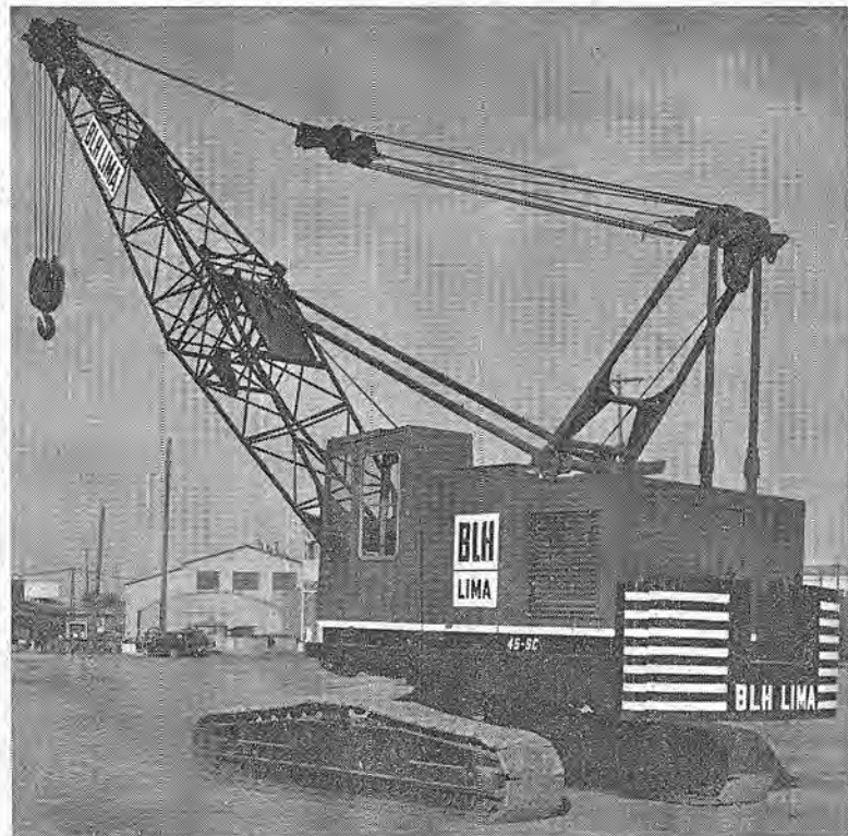
OVERALL SHOT of new 45-SC crawler crane built by Baldwin-Lima-Hamilton and boasting a number of outstanding new safety and environmental features for the operator. New crane is one of two that offers a breakthrough in pre-engineered safety and environmental health features that have been sponsored by union leaders for the past few years.
