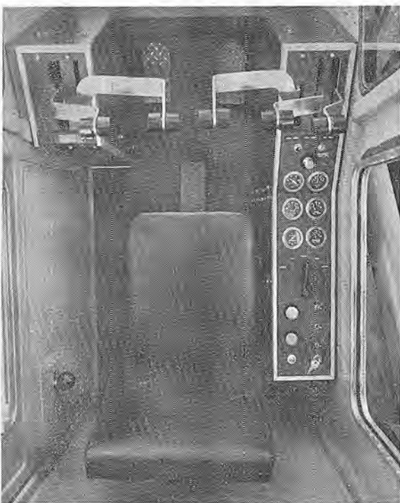
INTERIOR CAB SHOT of the new Baldwin-Lima-Hamilton 45-SC Crawler Crane that is the first to boast complete environmental cab control for the operator. Operator controls his environment with optional air conditioning and heating systems. Cab shuts out cold, heat and noise and boasts a four-way adjustable seat.
