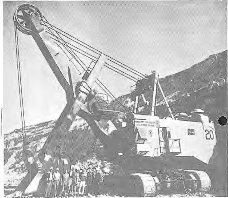
A FULL VIEW of the Marion electric shovel operating at Kennecott Copper.
