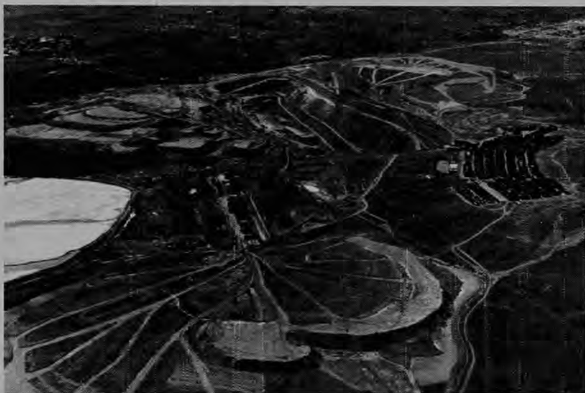
GIANT ANACONDA Open Pit and Plant at Weed Heights, Nevada which is 6,200 ft. long; 2,500 ft. wide and 700 ft. deep has turned loose 267,408,000 tons of ore and waste since going into
