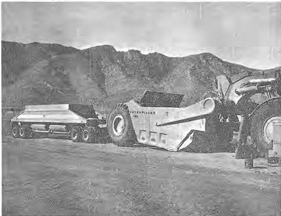
TWO KEY PIECES of equipment being used on the Burmiester-to-Timpie highway job in Utah are the 651 Scaper and 24-yard Trailer (left) and a new "Wheel." Fife Construction is the prime contractor on the job. Reports on the MX Wheel say that it has
