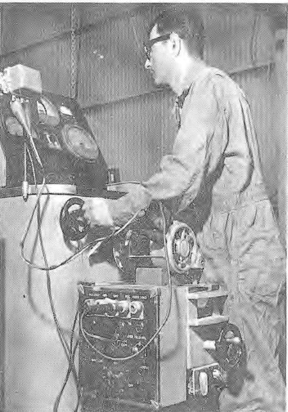
ALTERNATOR CHECK on a rebuilt Cat truck engine is tested by Brother Ernie Fierro in the Exchange Department of Peterson Tractor Company.
