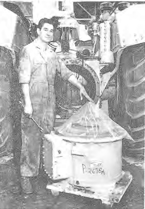
CAT 631 is about ready to get an exchange transmission at the Peterson Main Shop and Brother Len Ayala will do the honors on the tractor-scraper.
