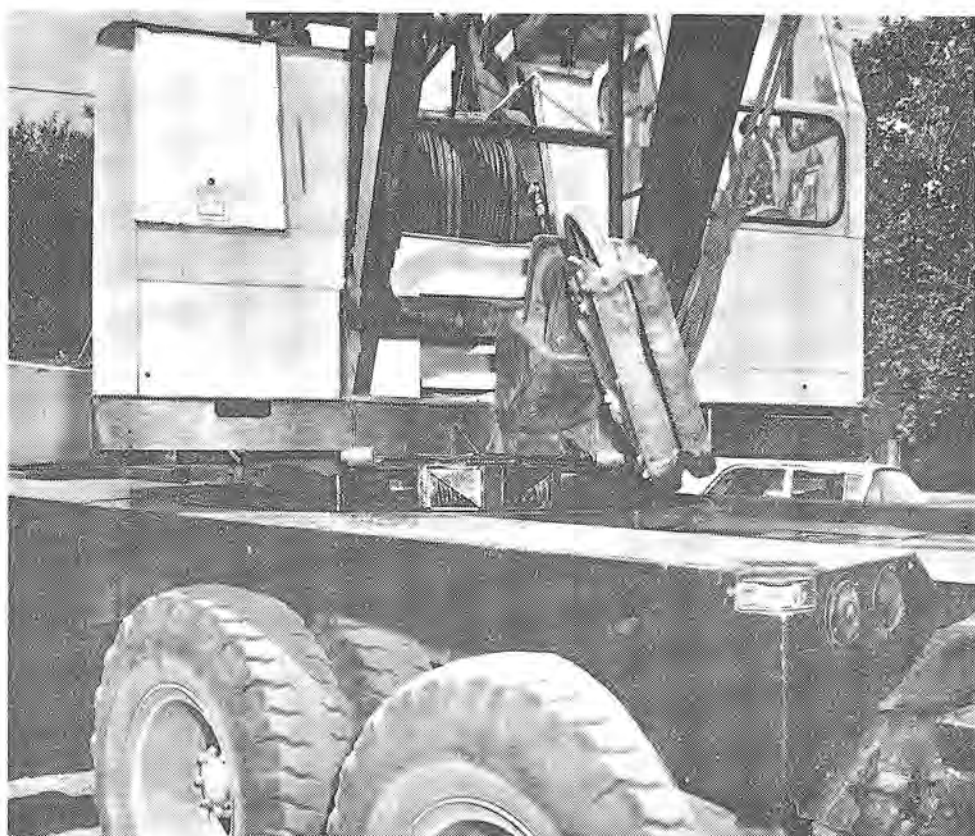
TWO VIEWS of new Boom Travel Limiting Device invented by Bob Ely.
