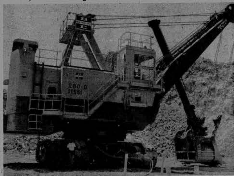
PICTURED IS a new Bucyrus Erie 280-B 15 yard electric shovel currently in operation at the New Melones Dam.
