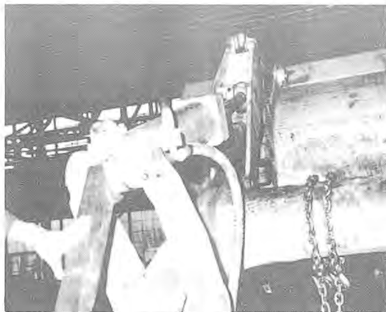
Steel braces between actuator and trunnion, and wood block under brackets prevent loader from falling during repairs to equipment.
