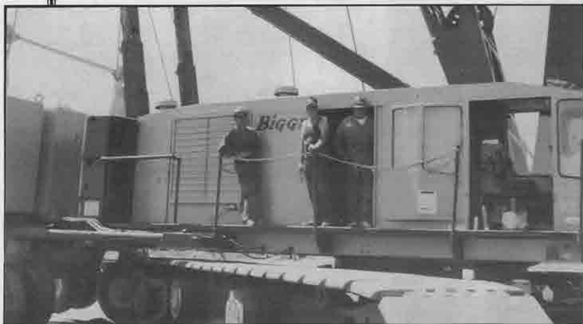
Right: Biggie Crane and Rigging recently moved in one of the largest cranes ever used in the Fresno area to move 19 bridge beams for the Hwy. 180 "Gap" freeway project. The crane was an American 1125 with a 600-ton lifting capacity. The Skyhorse on the rear of the crane weighed 200 tons. The 19 beams, which took three days to move into place, weighed 238,000 pounds each and measured 134 feet in length. Above: the crew was from left oiler Jay Brown, operator Randy Burke and mechanic Ken Bacon.
