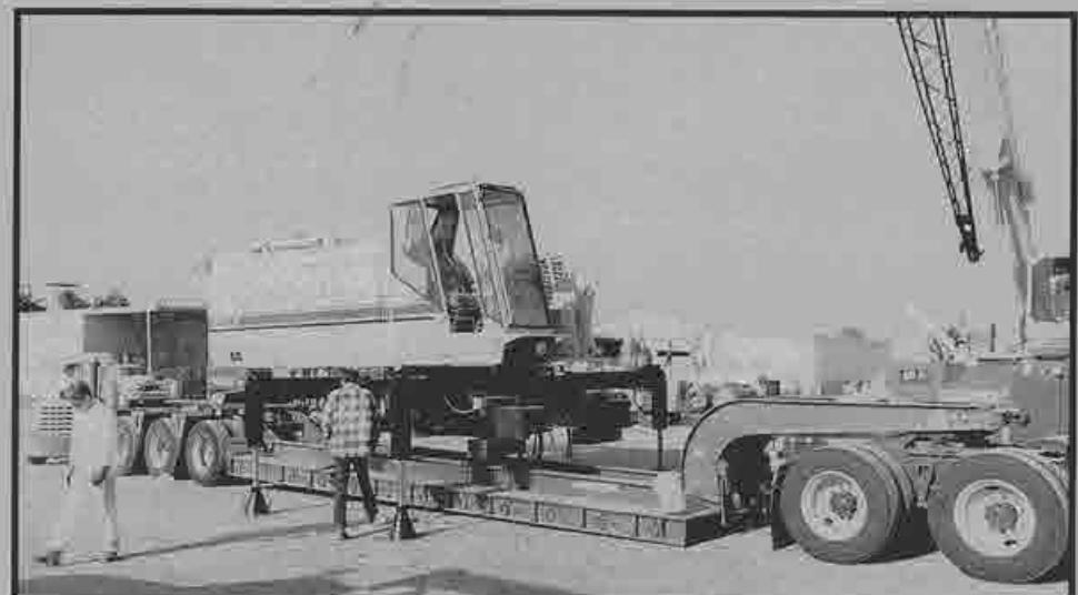
Right: After this LinkBelt LS 218H 100-ton crawler crane was delivered to Western Traction, Local 3 mechanics outfitted the rig for drilling and pile driving for Peter Kiewit Construction.
