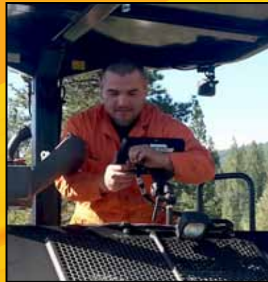
Heavy Duty Repairer (HDR) Albino Espinoza installs the display for the CCS 900 on a roller for George Reed.
