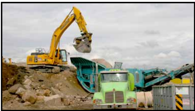
Operator Andy Mannisto loads debris into the portable asphalt crusher at Teichert’s Hallwood Plant near Yuba City.
